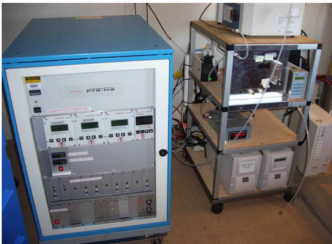
Figure C.1 The PTR-MS (left) and the associated zero and calibration gas dilution system (to the right) at the Boundary Rd site during the Wagerup Winter Study.
