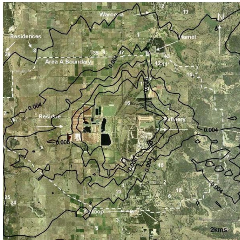
Figure 47: Peak (99.9 th percentile) 1-hour mercury concentrations for the existing (top) and expanded refinery (bottom) scenarios
